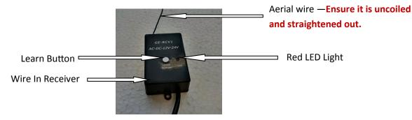
Press and release the LEARN BUTTON on the receiver and the Red LED light will glow on.
