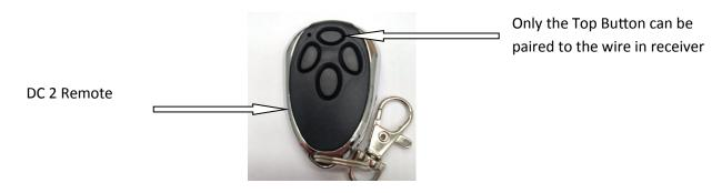
While the Red LED is glowing, press and release the top button only on the remote. The Red LED light will flash around 3—4 times and glow solid then go out.
