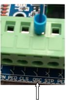
On the gate motor circuit board, connect the BLUE trigger wire to the OSC terminal.
