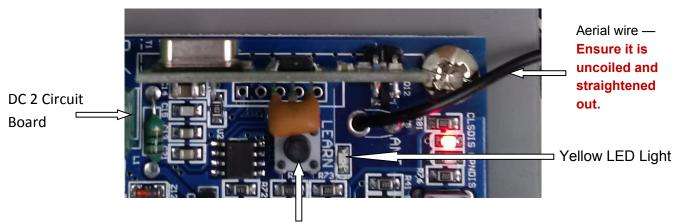
Press and release the LEARN BUTTON on the circuit board and the Yellow LED light will glow on.
