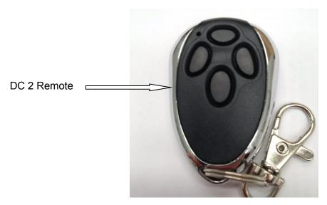
While the Yellow LED is glowing, press and release the desired button on the remote. The Yellow LED light on circuit board will go out.
