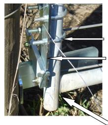
U bolts attach the latch mounting plate to the frame of the farm. Latching flipper plate
