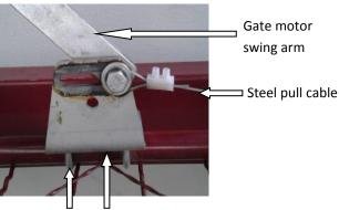
U bolts attach the mechanical latch gate bracket to the frame of the farm gate.
